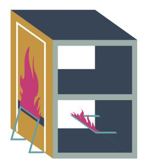
**3** Externally, flames shall not reach 10 feet above the window's top.
