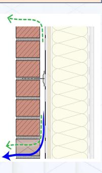
Specific detailing for cavity that allows drainage and venting or ventilation behind cladding. Larger capillary break and intentional airflow behind cladding. Degree of ventilation can be defined by an air exchange rate.
