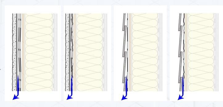
Specific detailing for drainage cavity to exterior. Drainage effectiveness can be measured per ASTM E2925-19A. Some degree of <u>venting can occur in some build-ups though is unintentional</u> and is a differentiator between a drained only vs rainscreen wall
