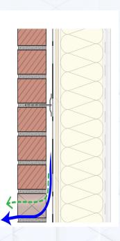
Specific detailing for cavity that allows drainage and venting or ventilation behind cladding. Larger capillary break and intentional airflow behind cladding. Degree of ventilation can be defined by an air exchange rate.
