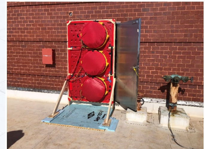
Photo 4 – Bank of Fans Installed in the Penthouse Door
