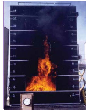
Full-scale Fire Test UBC 17-6 / UBC 26-4
