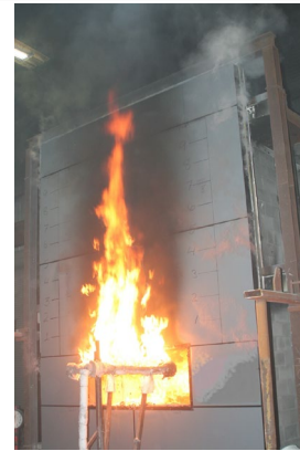
Reduced-scale Fire Test UBC 26-9 / NFPA 285
